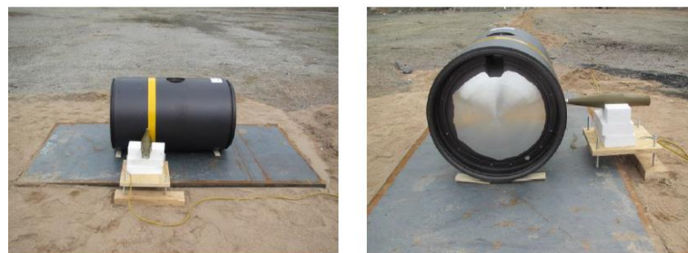
Figure 4 : Trial configuration : test specimen and RPG-7 shaped charge
