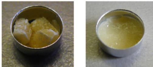
Figure 5: MC-1 in a DSC cup, left side before melting, right side after melting
