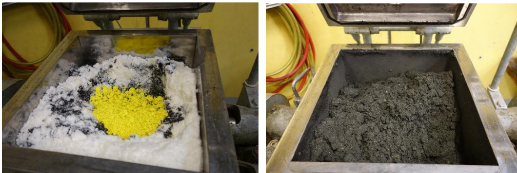
Figure 6 Paste before and after final step of mixing. Pre-mix with additives (black), pre-mix without additives (white) and FOX-7 (yellow).
