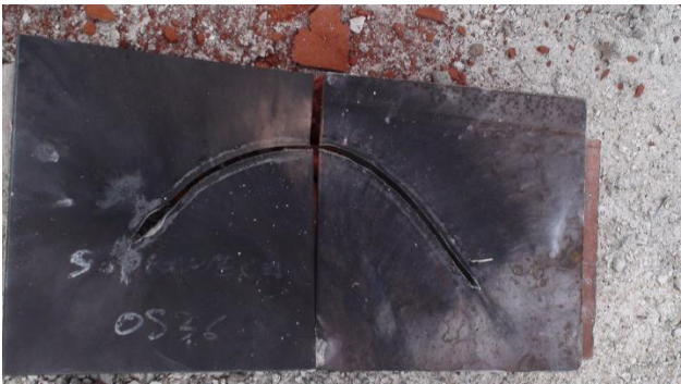
Picture 12: Cut steel plate after ignition
