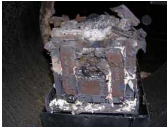
Picture 6: Hexomax in logistic plywood box after slow cook off
