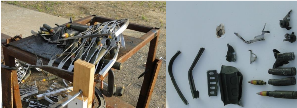
Figure 9: Test stand post-test, showing scattered aluminum trays and rounds (left); Post-test debris that traveled farther than 50 ft (right).
