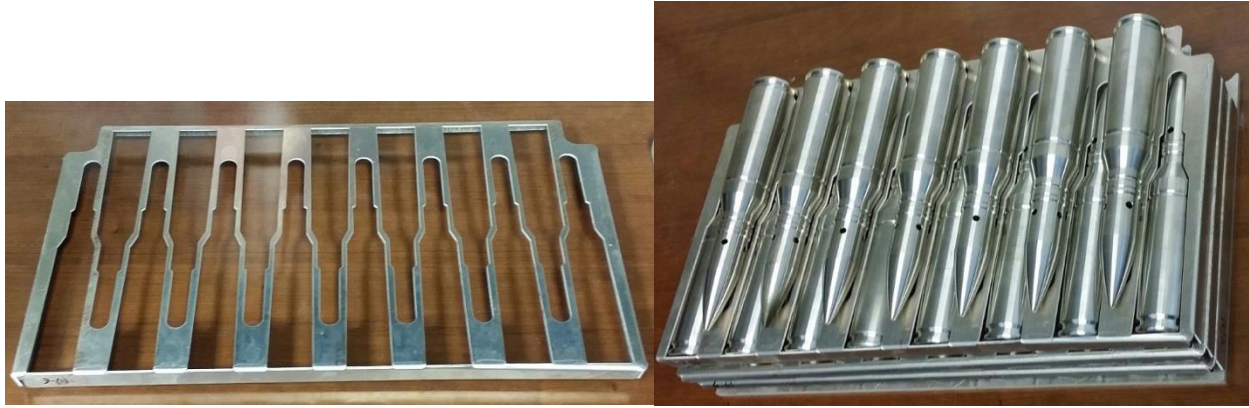
Figure 2: Prototype aluminum tray (left); Three trays stacked with dummy 25mm rounds (right)
