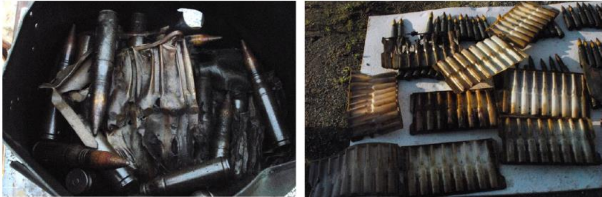
Figure 3: Comparison of plastic tray thermal degradation from Test 1 (left) and Test 2 (right)
