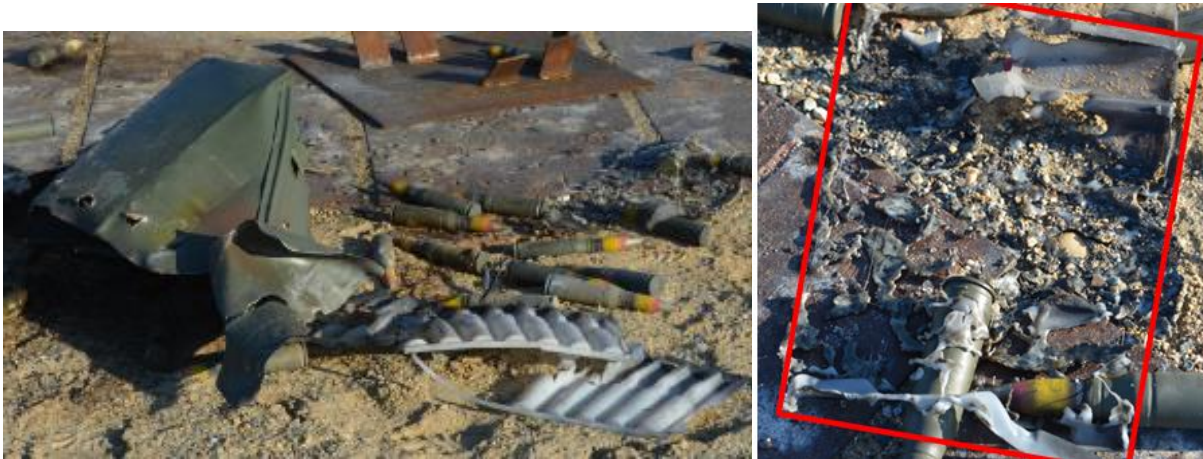
Figure 6: Post-test debris of BI Test 5 showing catastrophic damage to the ammo can (left) and a burned HDPE packing tray (right)
