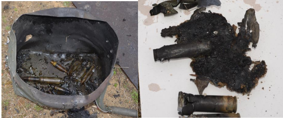
Figure 7: Remains of cooked-off rounds and burned trays (left); A partially burned tray fused to empty cartridge case (right)
