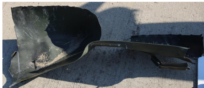
Figure 8: Ammo can post-test, completely blown open
