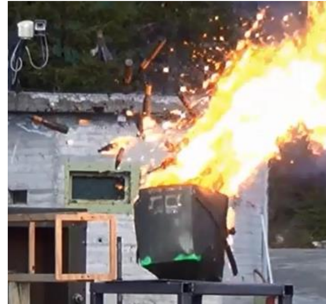
Delayed Cook-off Reaction due to burning HDPE trays
