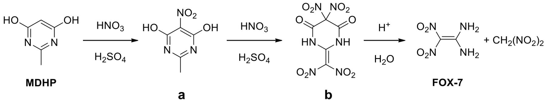
**Mixed acid nitration conducted at 10-30°C**
