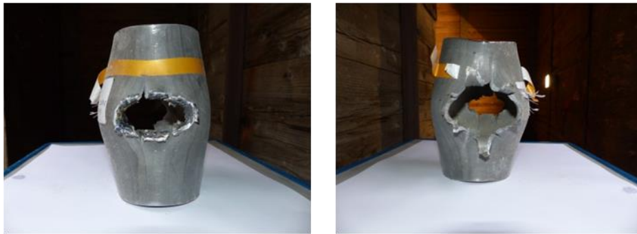
Fig. 8: Steel casing of test V-13943 with ERL = VI: entry side (left) and exit side (right).
