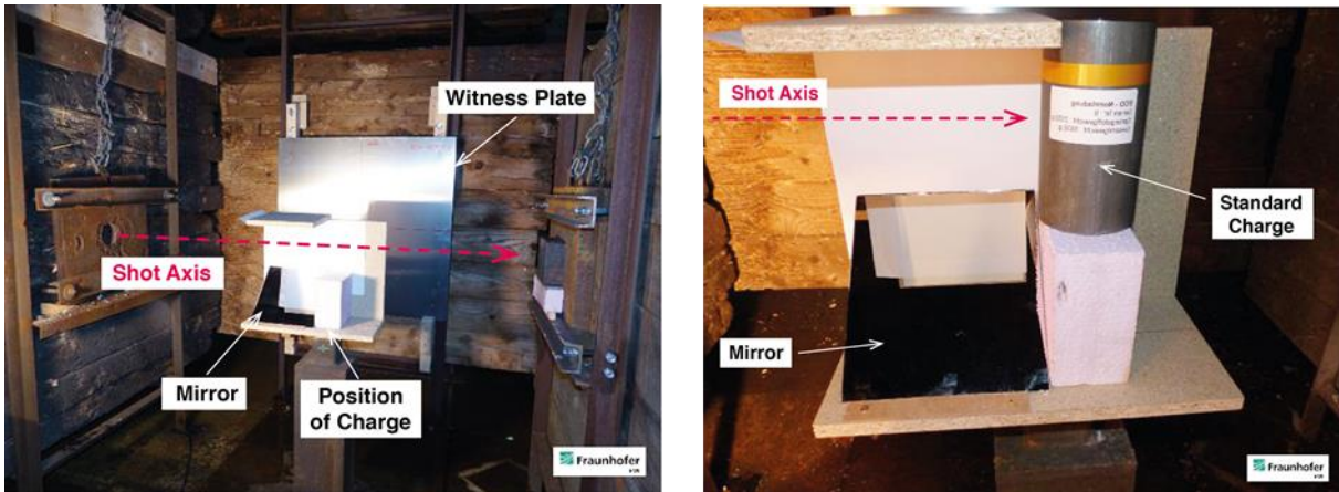
Fig. 5: Test setup at the EMI impact chamber (left) and a close-up of the TDW standard charge (right).
