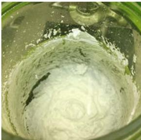
If lacquer was added to a warm (60 °C) slurry, the binder becomes associated with the water phase and coats the vessel rather than forming beads.
