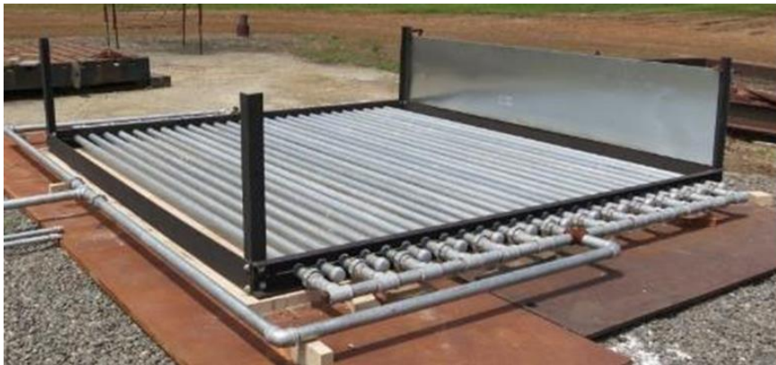
Figure 1. US Navy FCO 3.7 m by 3.7 m propane burner located in Dahlgren, Virginia
