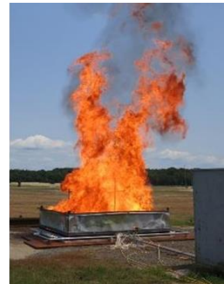
Figure 1. US Navy FCO 3.7 m by 3.7 m propane burner located in Dahlgren, Virginia
