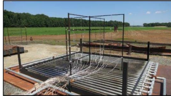
Figure 7. Burner calibration arrangement and test
