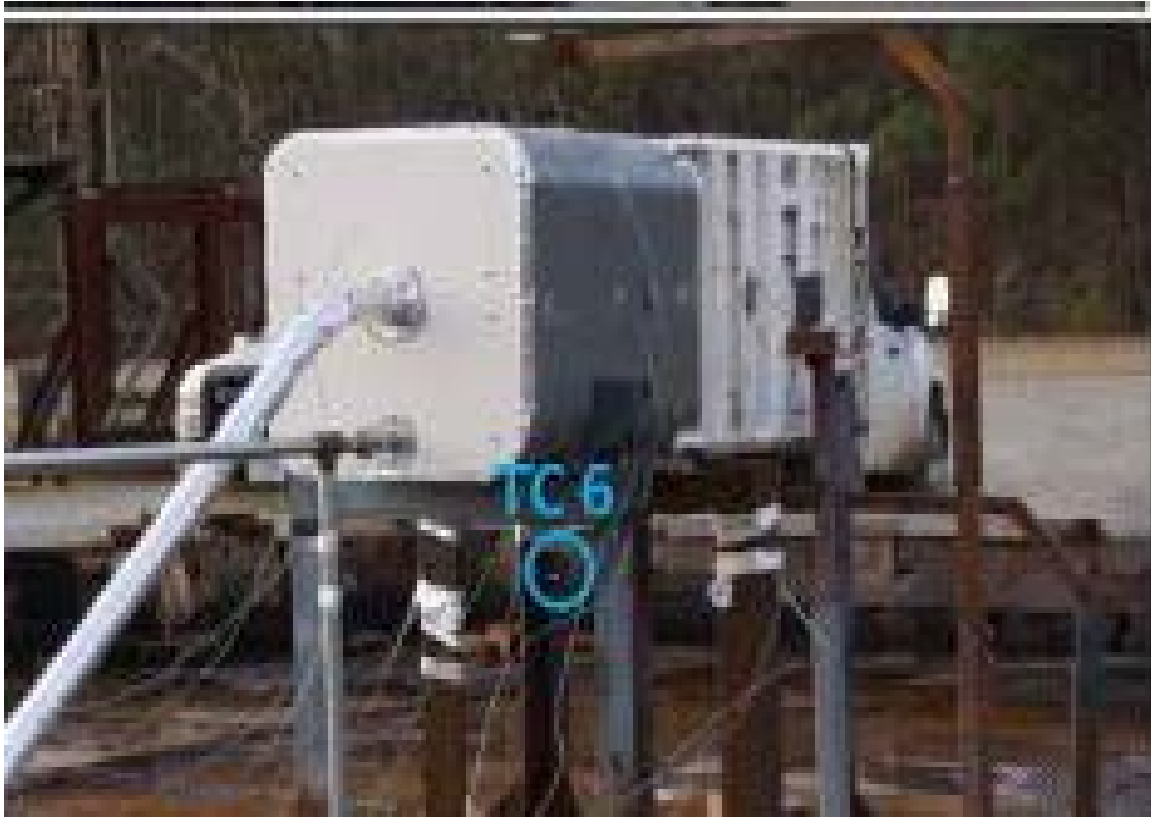
Figure 2. Thermocouples on canisters.
