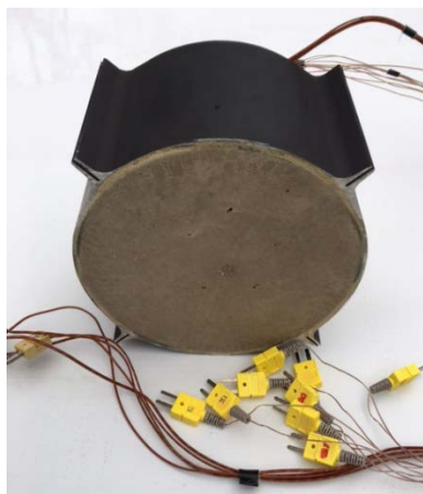
Figure 14. Interior instrumentation showing thermocouples to measure the temperature at the interface between the insulation and propellant.
