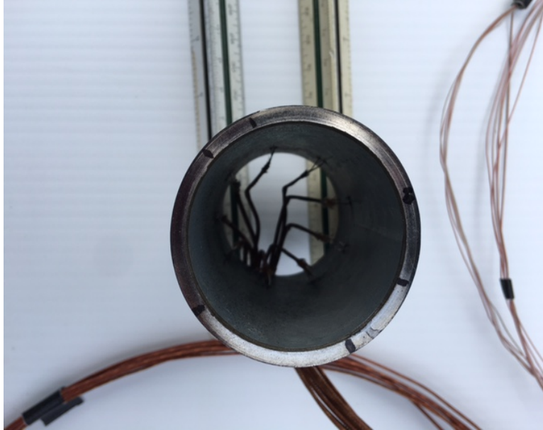
Figure 4. Calorimeter for showing angular uniformity of temperature. Thermocouples are welded to the calorimeter at nine locations around the inner circumference.
