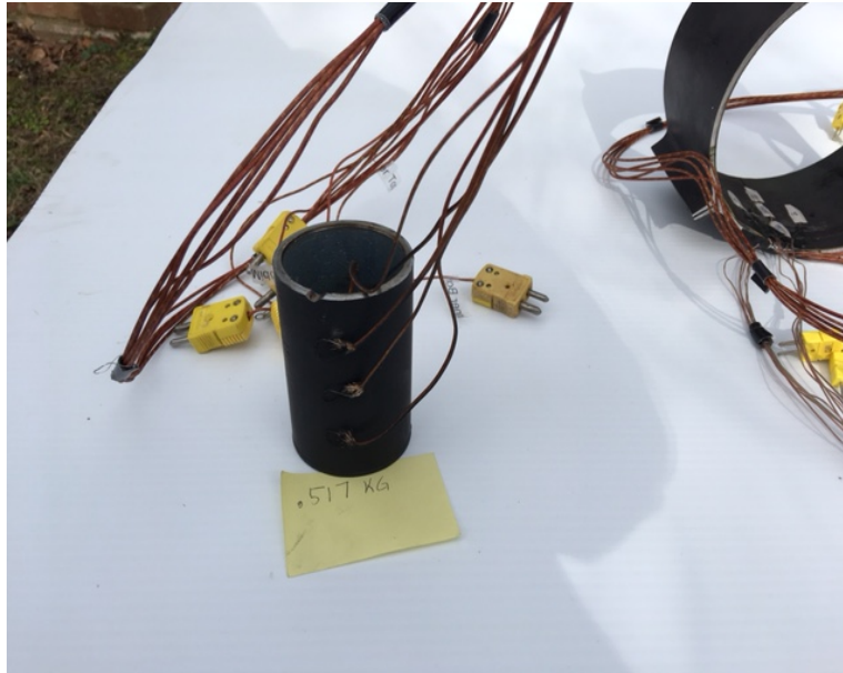
Figure 6. Calorimeter for calibrating heat flux and showing uniformity of temperature and heat flux. Three axial stations were monitored on both surfaces of the calorimeter.
