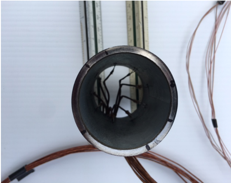
Calorimeter for showing angular uniformity of temperature
