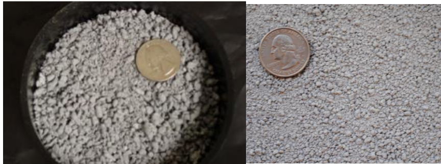
Figure 1: Granules of PAX-3 produced in a twin screw extruder (left) and slurry process (right)
