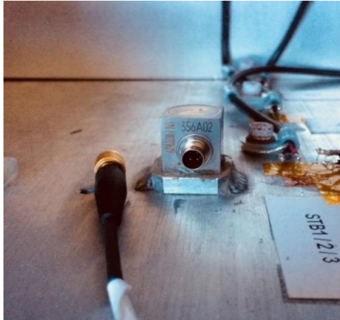
Triaxial accelerometer mounted to welded stud plate inside witness object
