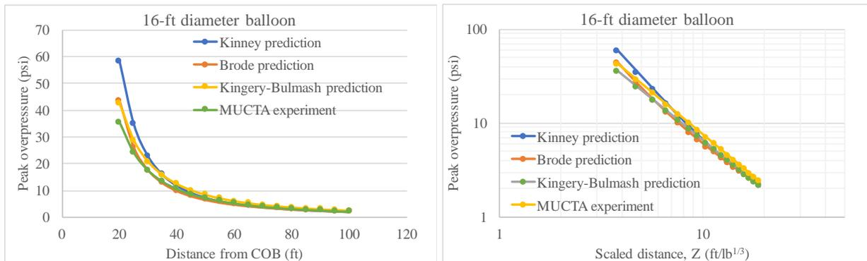
**Figure 7.** Comparison of experiment with TNT prediction for a 16-ft. diameter balloon gas mixture (left) Peak overpressure variation with distance (right) Log-log plot of peak overpressure variation with scaled distance
