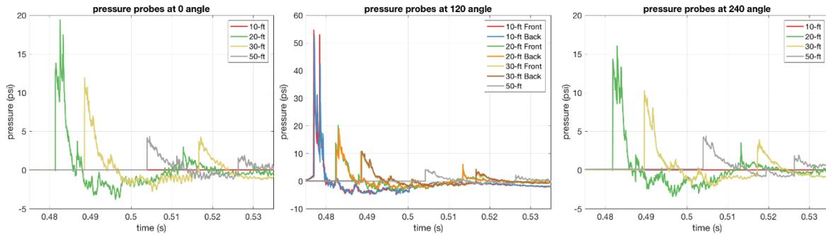
**Figure 3.** Typical pressure time history from a 12-ft. diameter balloon explosion
