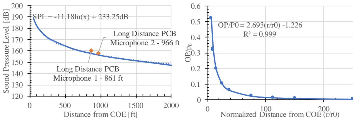
**Figure 11.** (left) Sound pressure level (SPL) acoustic decay model with distance indicating the measured acoustic data points. (right) Normalized overpressure decay with normalized distance in the acoustic regime
