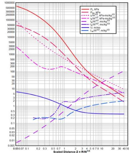
**Figure 5.** Parameters of positive phase of shock spherical wave of TNT charges from free-air bursts [6]
