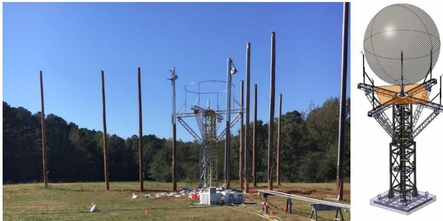
**Figure 1.** (left) Central balloon tower with pressure probes installed on poles (right) CAD snapshot of central test stand with 16-foot diameter balloon
