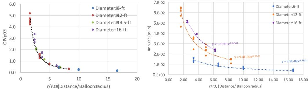
**Figure 4.** (left) Normalized Overpressure variation with normalized distance (right) Average impulse variation with normalized distance
