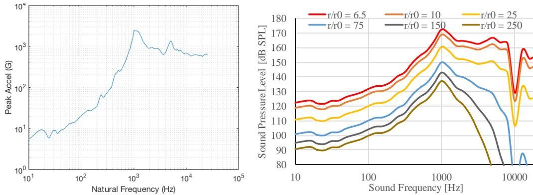
**Figure 10.** (left) Shock response spectrum of 16-ft diameter balloon CH<sub>4</sub>-GO<sub>2</sub> blast event at 50 ft. from COE (right) Distribution of the frequency from the blast overpressure with distance normalized with balloon radius  $R_0 = 8$  ft.
