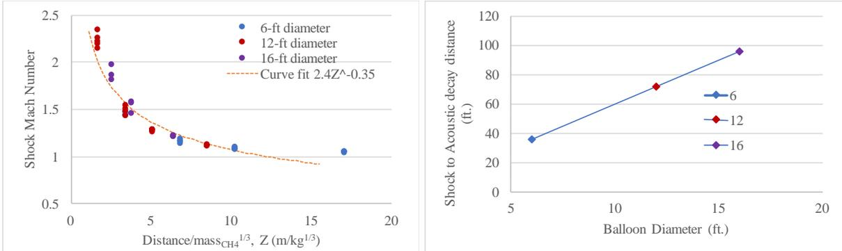
**Figure 9.** (left) Mach number variation with normalized distance (right) Approximate shock to acoustic decay for different balloon sizes based on the Mach number approach
