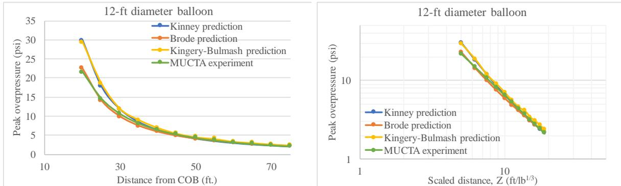
**Figure 6.** Comparison of experiment with TNT prediction for a 12-ft. diameter balloon gas mixture (left) Peak overpressure variation with distance (right) Log-log plot of peak overpressure variation with scaled distance
