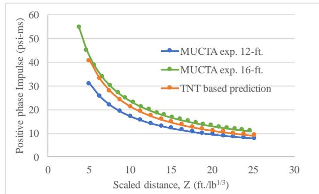
**Figure 8.** Comparison of impulse data from experiment with TNT predictions
