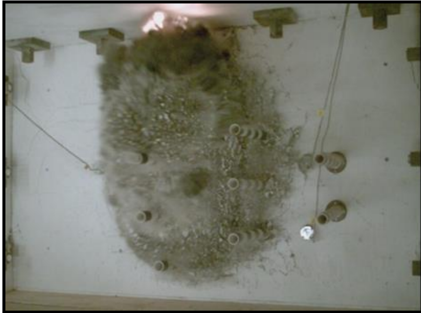
Wall 1 breach: snap from test Video
