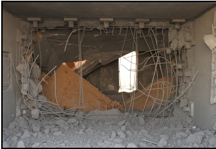
Internal view of test wall 1
