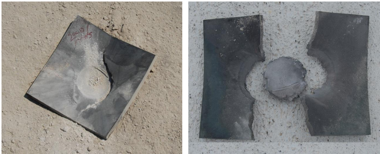
Figure 4. Witness Plates From 2-inch-diameter (left) and 2.25-inch-diameter (right) Critical Diameter Tests
