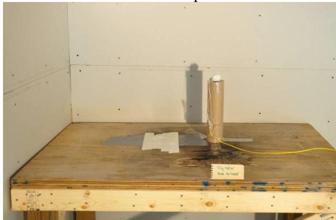
Figure 2-3 – Test 8, 50 g Total Net Explosive Weight (NEW) Non-Containerized Bare Explosives
