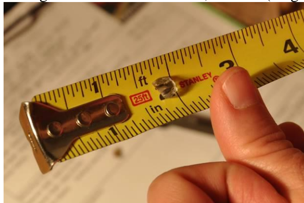
Figure 2-6 – Largest Glass Beaker Debris, Test 10 (10 g total NEW)
