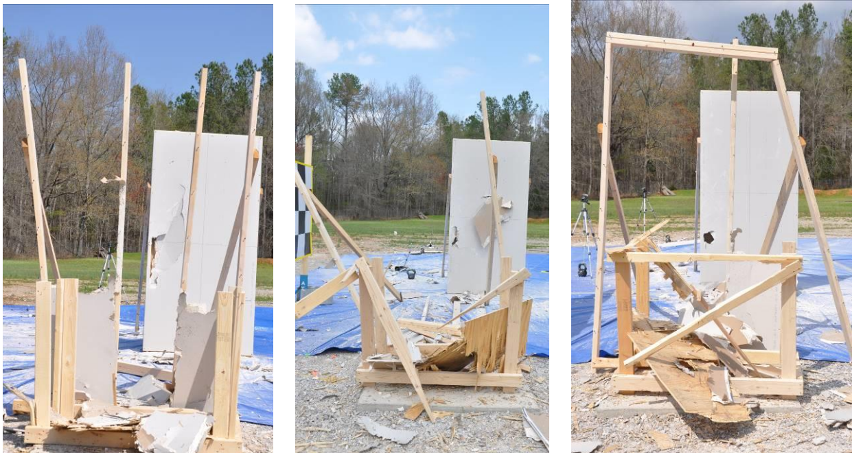
Figure 3-3 – Typical Damage from SQRL Phase II Test Series 2 (250 g C-4, 12” Stand-off)
