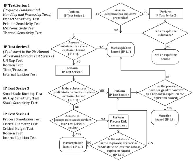
Figure 2: Energetic Substances Classification Decision Tree for In-Process (IP) Operations
