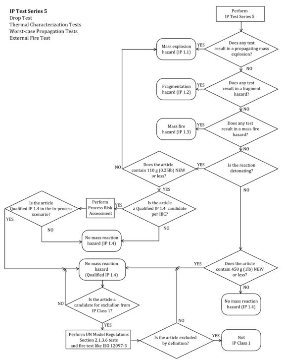
Figure 3: In-Process Article Classification Decision Tree for In-Process (IP) Operations
