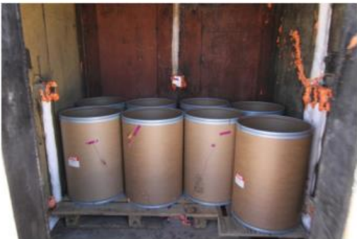
FIGURE V-1. Test 4 Structure With M1 Propellant Filled Barrels.
