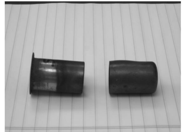
Photo 7: Koenen tube after Trial 4 AORC test with minimum surface area shows minor damage and break at score line.
