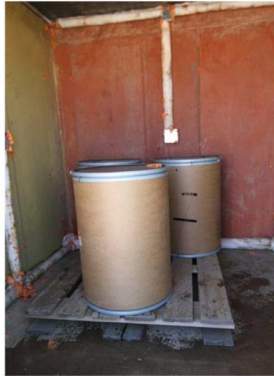
FIGURE I-6. Three Drums of M1 Propellant Placed Within the Structure for Test 1.
