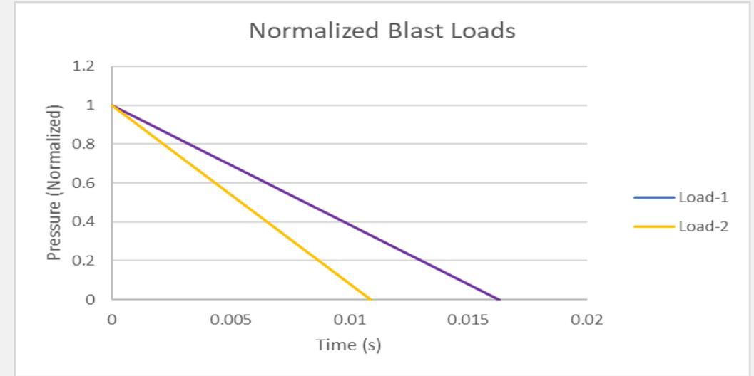
The structure dynamic response was given 100ms to settle after the gravity load was ramped up, and then at 500ms the blast load was applied
