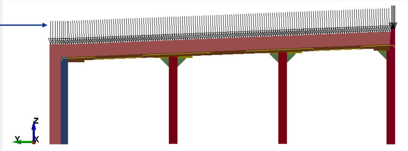
Simplified blast load allows comparison to previous SDOF studies and is required for design of magazines. This simplified load increases overall impulse seen during loading.
