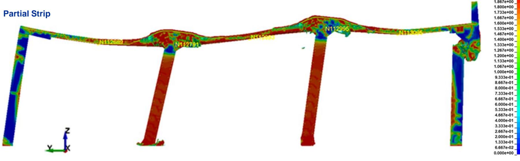
Partial strip model exhibited racking at late time (see figure to left) while half-symmetry model was stable. This indicates the importance of modeling the side wall which provides an additional membrane to tie the front and rear walls together.
