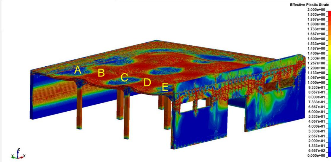
Roof slab nodal velocity settles at 0 in/s w/o roof slab being thrown in
