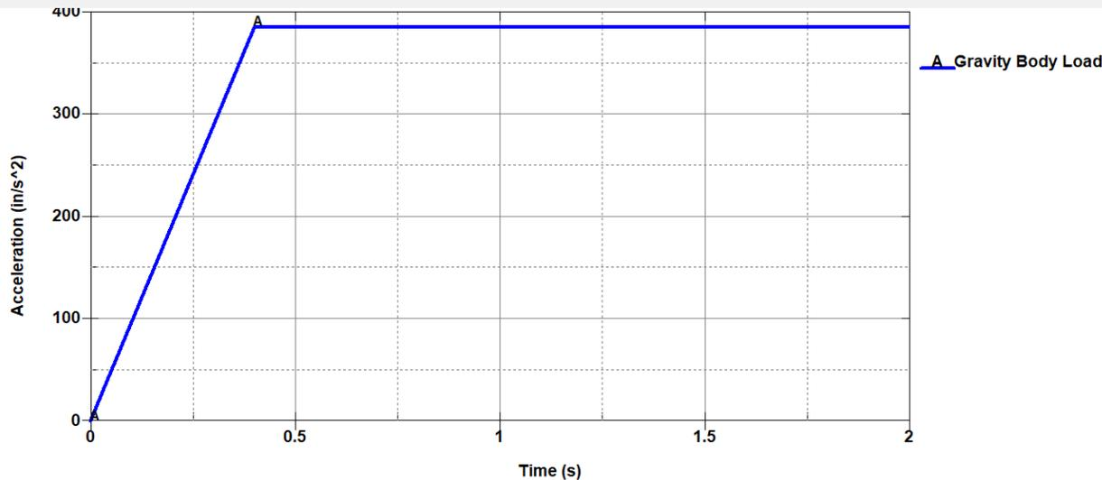
Gravity load was applied to all bodies, ramped up to 386.1 in/s<sup>2</sup> during the first 400ms of simulation, and then held steady
