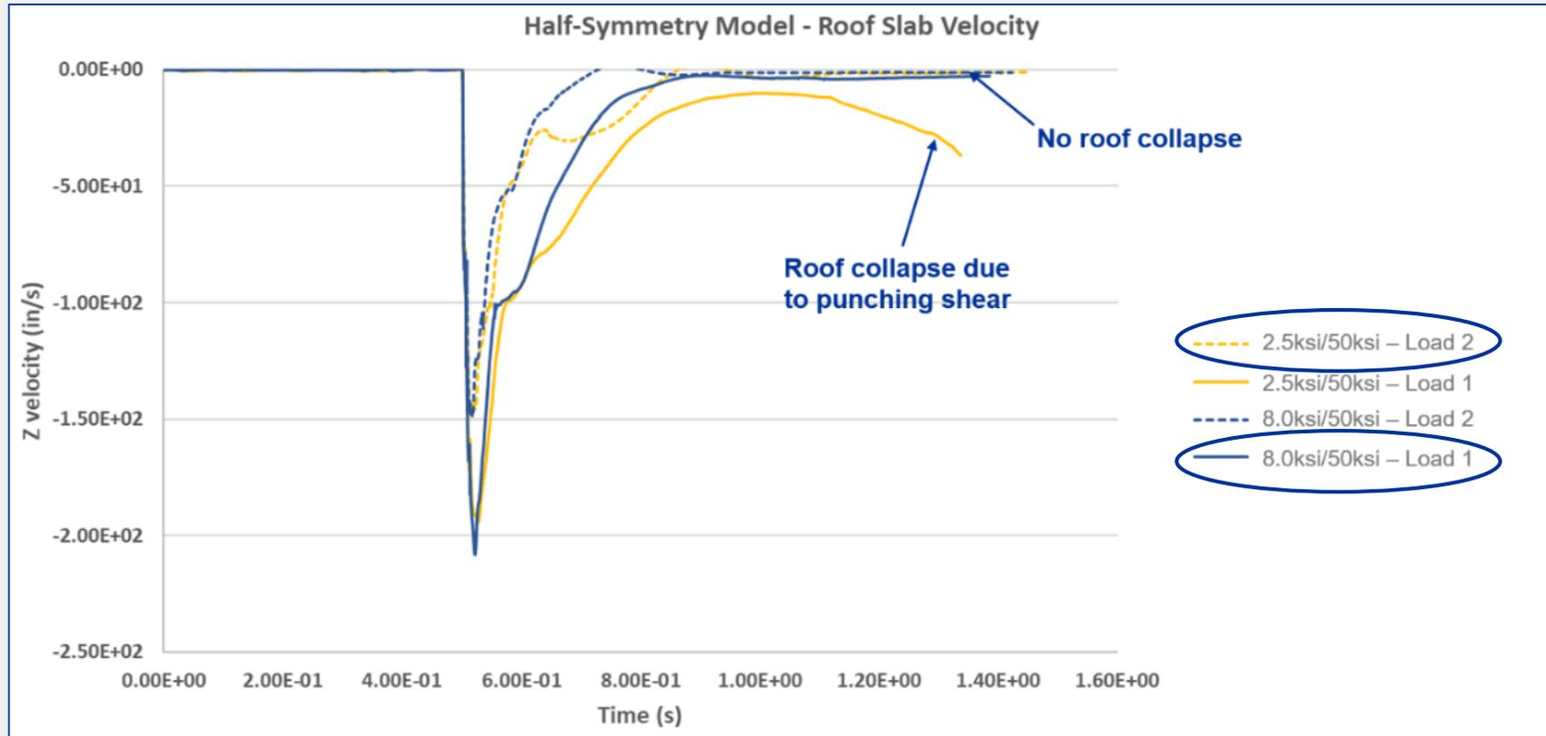
These cases showed instability and failure with the partial-strip model, but with the half-symmetry model showed stability and no roof collapse
