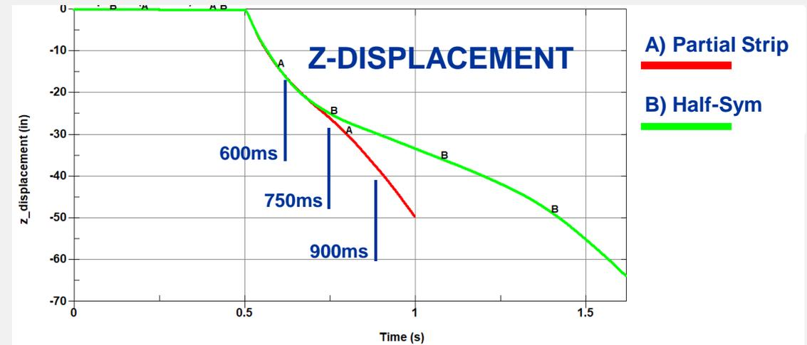
Half-symmetry model response begins to diverge from partial-strip model at approximately 700ms.
