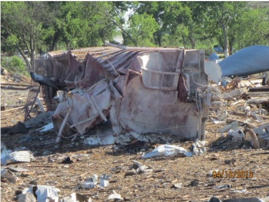
Figure 4. Rail Car Loaded with Ammonium Nitrate Overturned by Explosion
