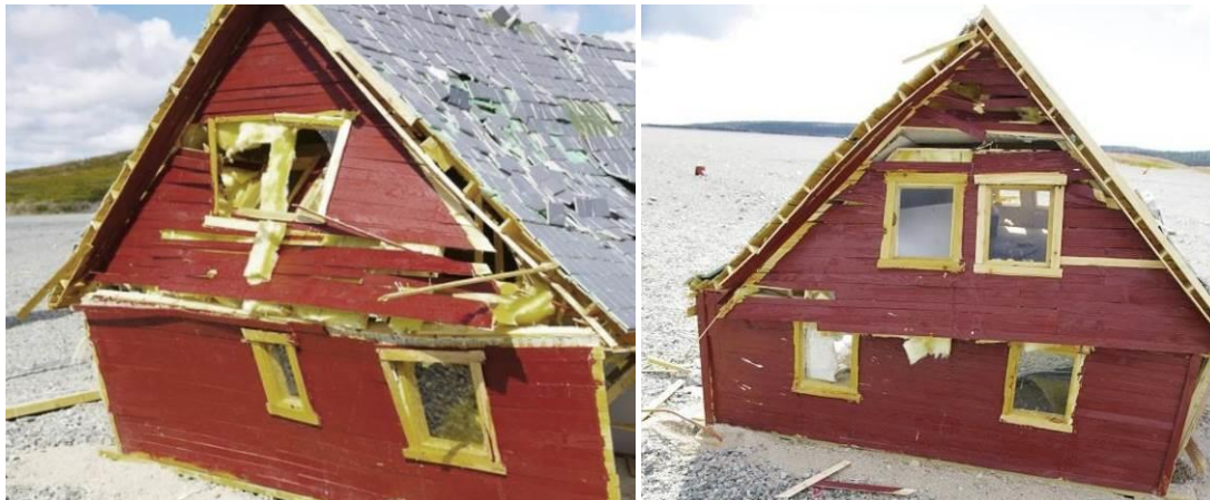
Figure 5 Gable walls of Lykkebo in scale 1:5 after detonation of 350 kg Texit 40 35 m from the house 15
