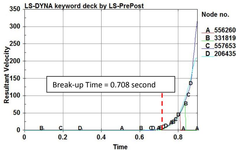
Figure 7: Break-up Time Determination with Resultant Velocities
