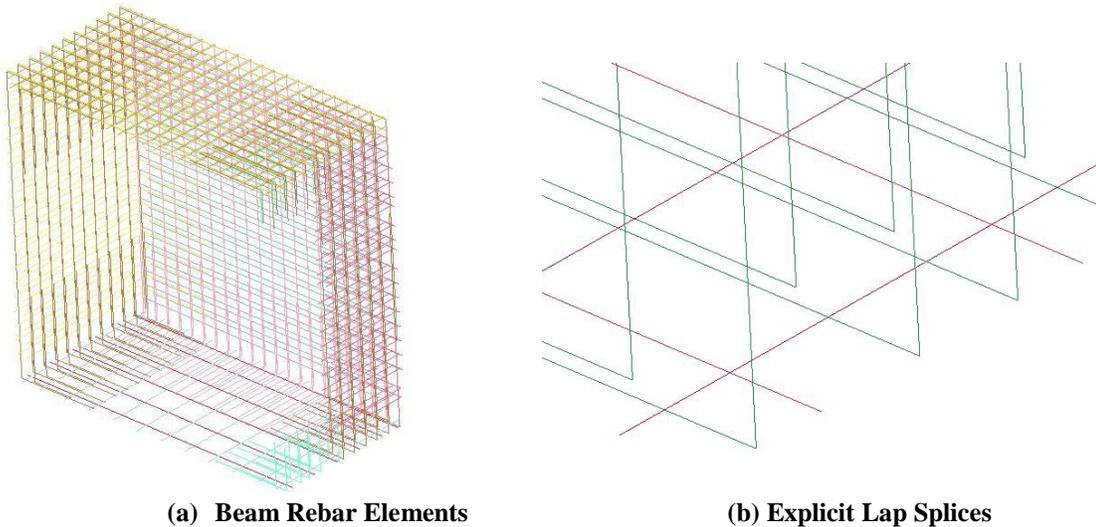
**Figure 3: Steel Reinforcement Modeling**
