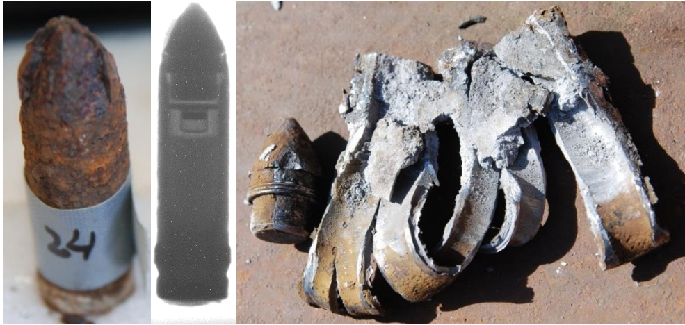
Figure 4. Example of UXO (20 mm armor piercing incendiary grenade) in vertical, fixed, “worst-case” position before mechanical testing (left), x-rayed (center) and after testing (right) (Menning, Carlsson, et al. 2014).
