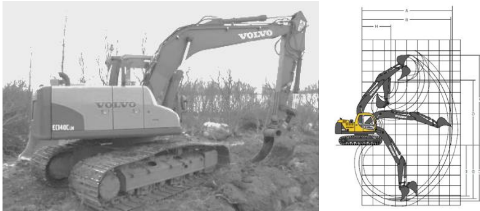
Figure 2. A representative excavator (Volvo EC140), combined with the maximum possible exerted force on UXO, was the starting point for designing a mechanical test equipment for translating the same mechanical influence (Menning, Carlsson, et al. 2014).
