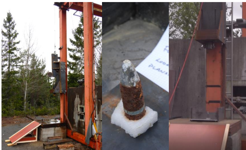
Figure 3. Deterministic, or “worst-case”, testing of mechanical influence on UXO (of 12.7 to 30 mm medium caliber ammunition origin) for determining hazardousness (Menning, Carlsson, et al. 2014).
