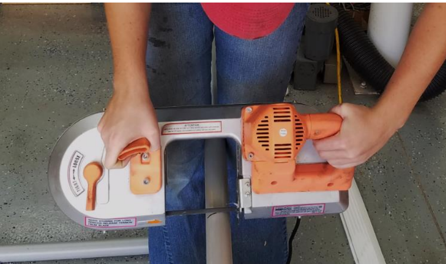
Portable bandsaw cutting DN 25 (1-in NPS) stainless steel pipe
