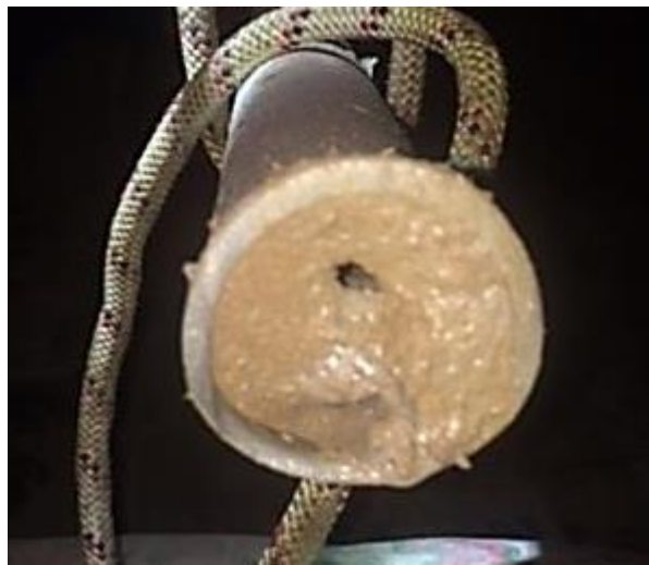
Figure 7 – Typical Comp A-3 Explosive Filled Pipe
