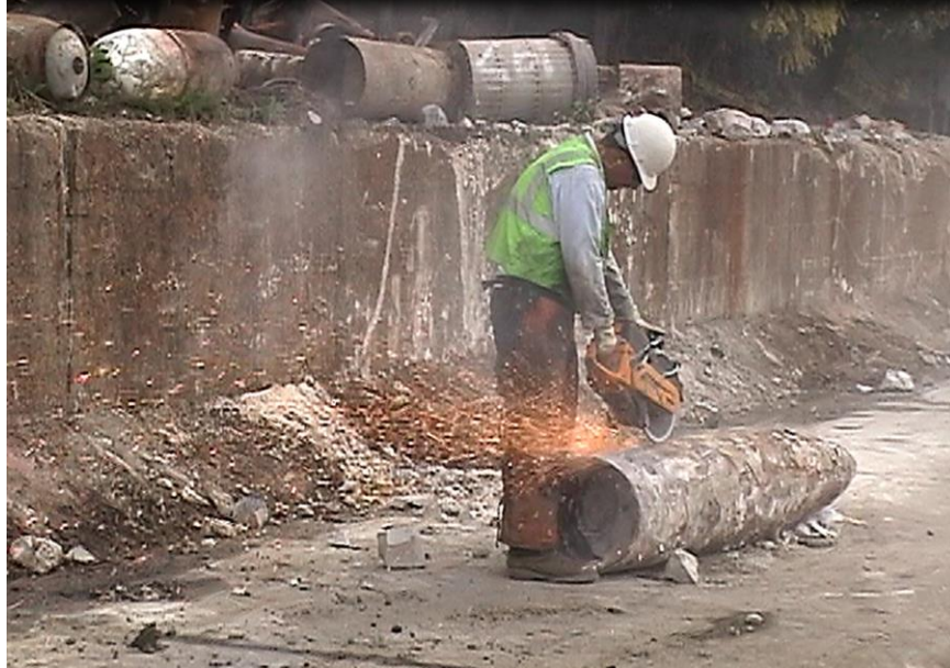
Figure 5 – Abrasive Saw Cutting Inert Bomb Skin
