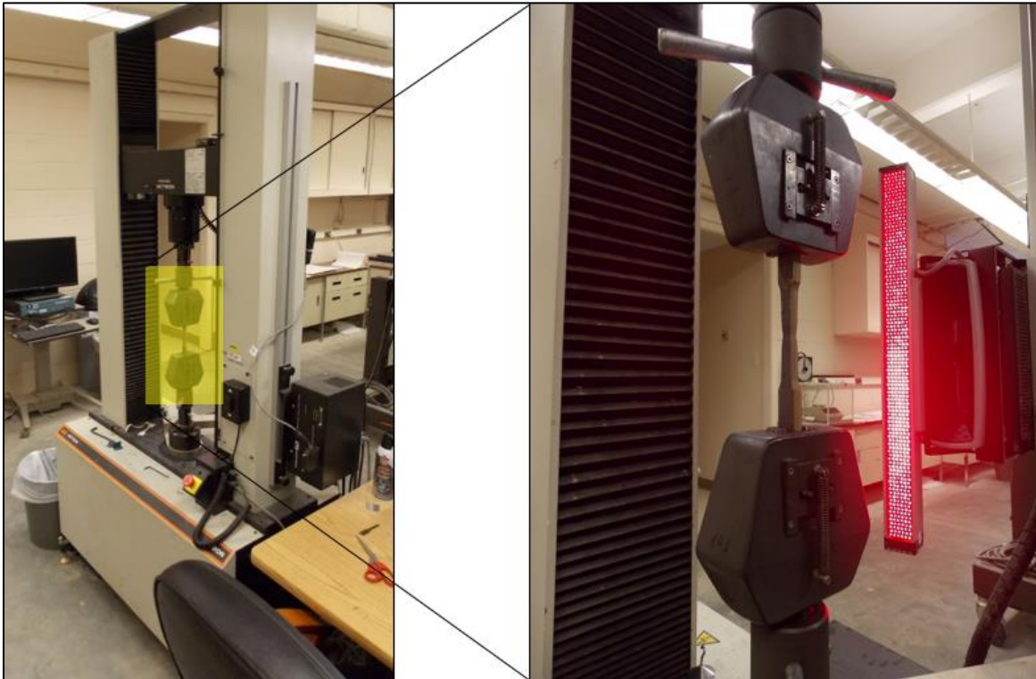
Figure 3. Instron uniaxial tension test machine used for static-rate testing.
