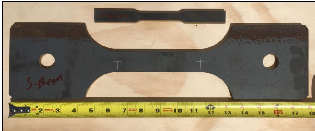
Figure 2. Static (top) and dynamic (bottom) uniaxial tension specimens.
