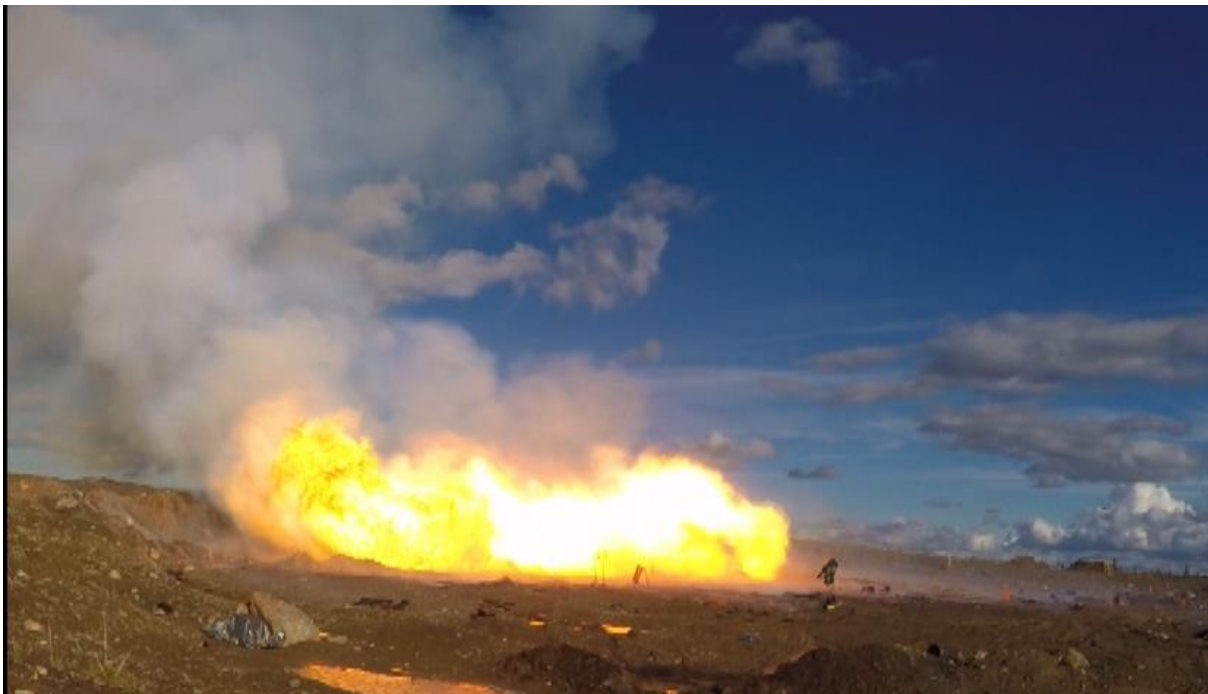
Figure 6. Finnish test containers after ignition of second container
