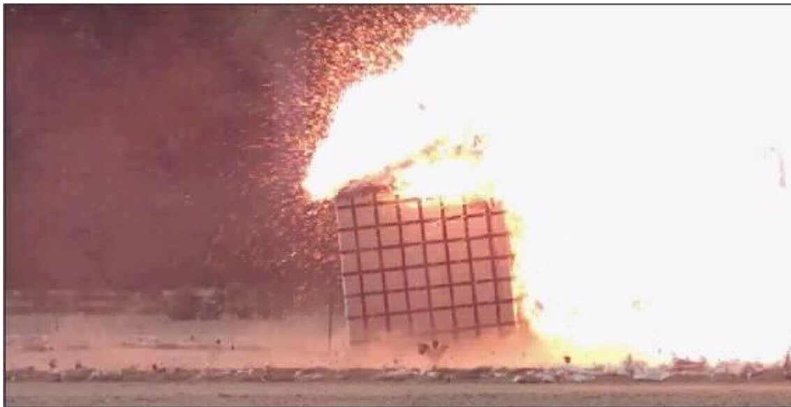
Figure 14. Image from DDESB test 4 with 503kg of propellant after rupture of structure
