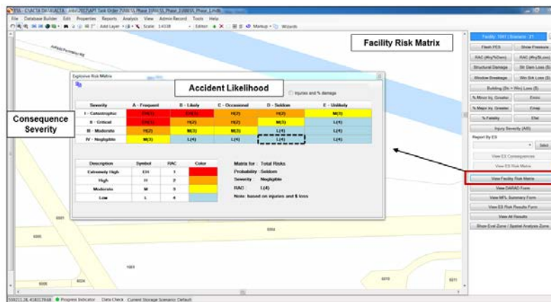
Figure 30. Tier 2a Analysis Results (Risk Matrix) (Displayed maps and data do not represent existing explosives sites).
