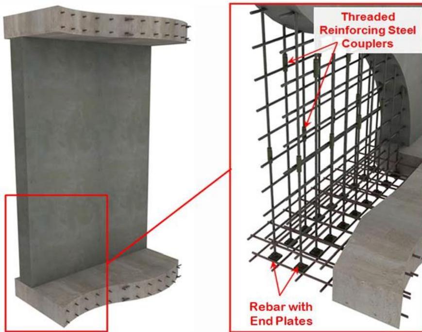
**Figure 1. RC wall with threaded reinforcing steel couplers and rebar with end plates**
