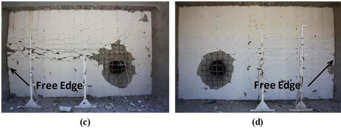
**Figure 6. Post Test 2 and 3 photos of non-loaded faces of walls (a) RC Baseline Wall; (b) RC Test Wall; (c) RC Baseline Wall; and (d) RC Test Wall**
