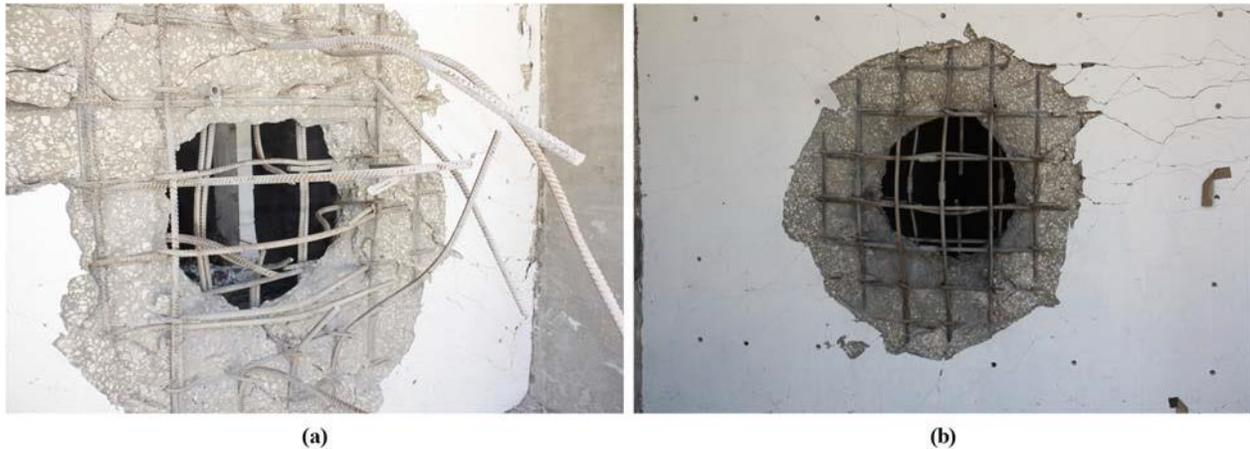
**Figure 10. Reinforcement details post Test 3; (a) Baseline RC wall; (b) Test RC wall**
