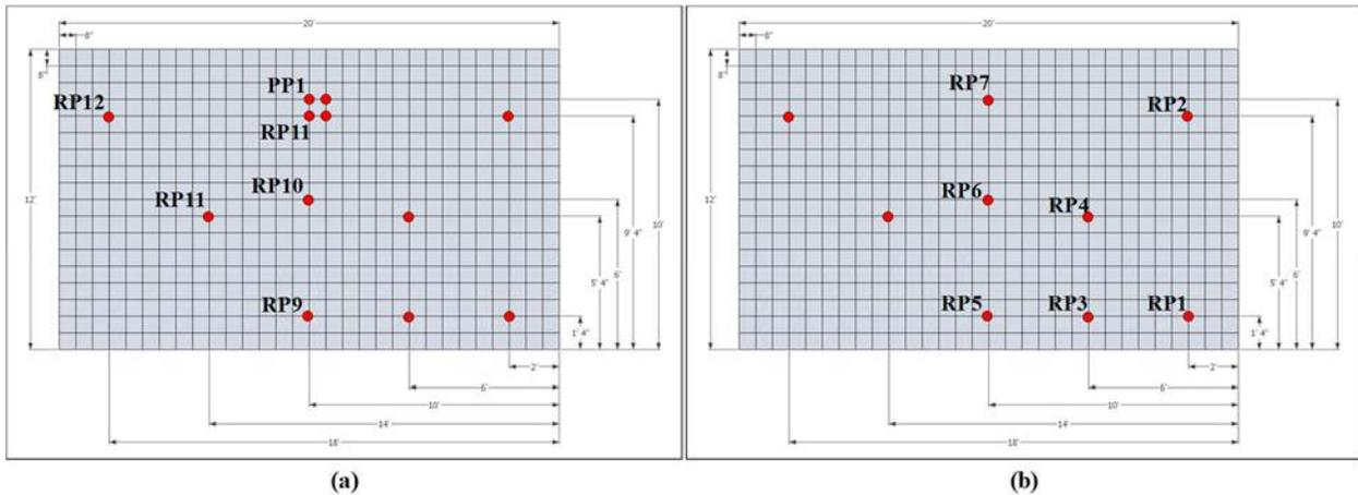
**Figure 4. Interior view of reflected pressure gauges; (a) RC Test Wall – rebar couplers and rebar with end plates; (b) RC Baseline Wall –conventional reinforcement**
