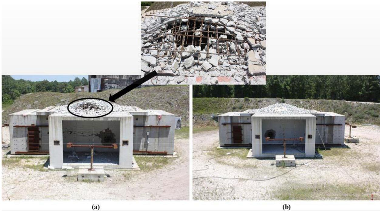
**Figure 11. Performance of roof system post Test 3; (a) Roof-wall connection for Baseline RC wall with callout to roof damage; (b) Roof-wall connection for Test RC wall**
