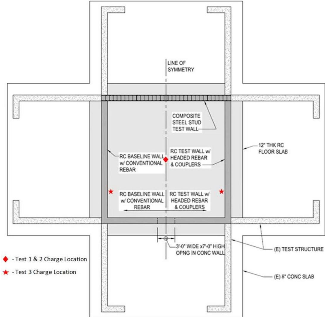
**Figure 3. Plan view of HIBS test setup**
