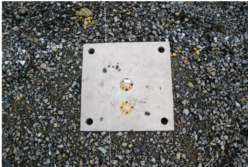
Figure 4 Surface-flush mounted pressure gauges in Test Series 2
