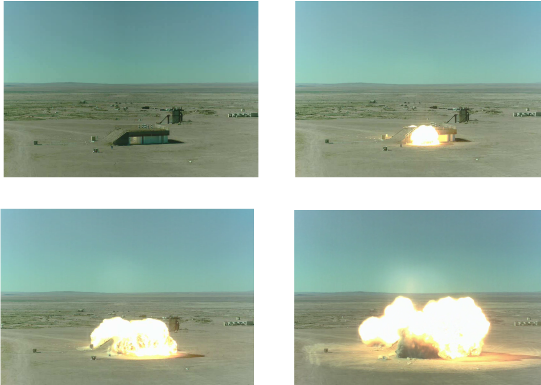
Figure 6 Still images from the explosive test showing blast wave and fire ball propagation
