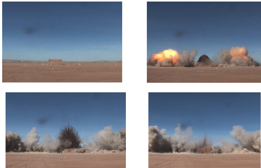
Figure 9 Still images from the explosive test showing the ejection of debris and soil from the roof of test structure
