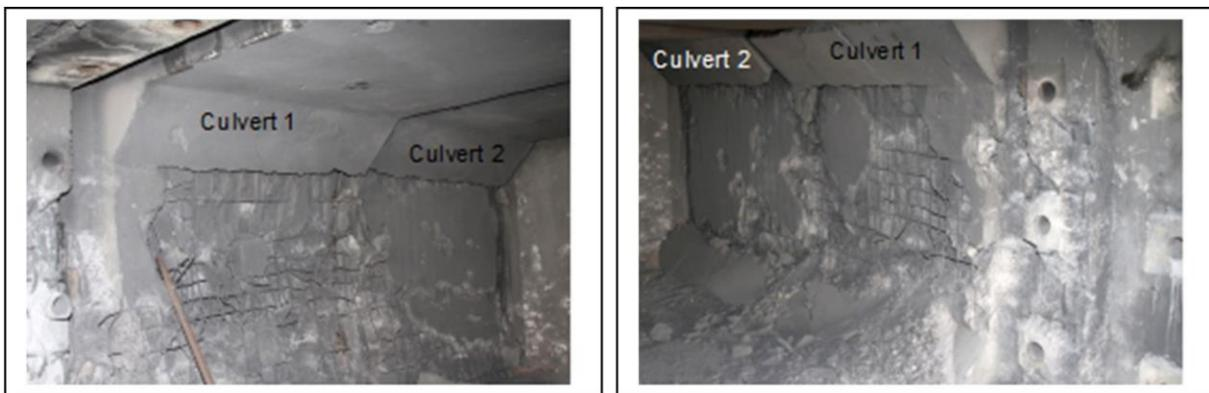
Figure 13. Test results show the significantly damaged east and west culverts.
