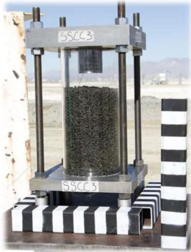
Fig. 1. Experimental setup. (6" diameter, 13" height polycarbonate tube filled with 7lb M1 gun propellant. 20g of Red Dot smokeless powder was filled in the steel basket on the steel lid).
