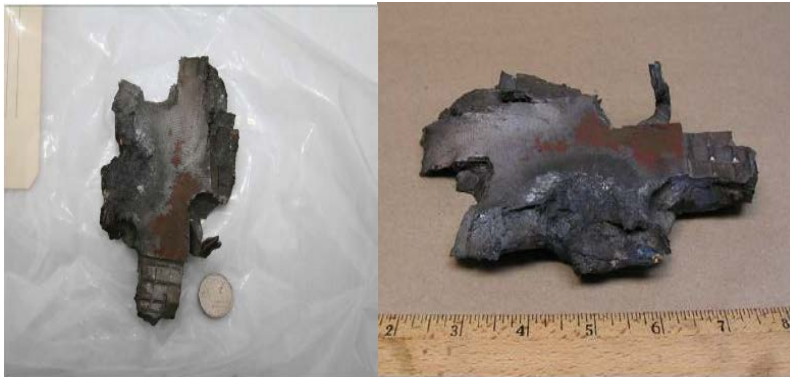
840 g steel fragment from a M107 155 mm artillery shell that reached 1824 m after a sub- detonative response. (Baker)
