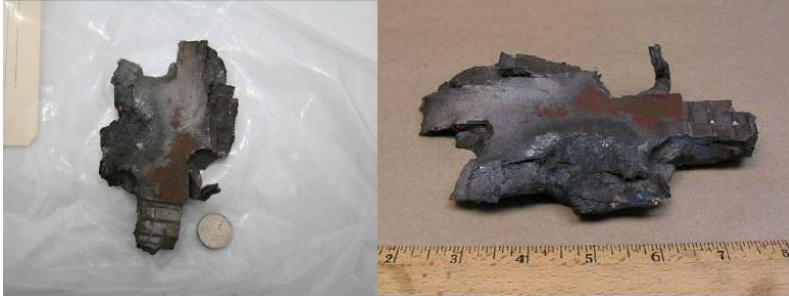
Figure 11 840 g steel fragment from a M107 155 mm artillery shell that reached 1824 m after a sub-detonative response [Baker, et al., 2009].
