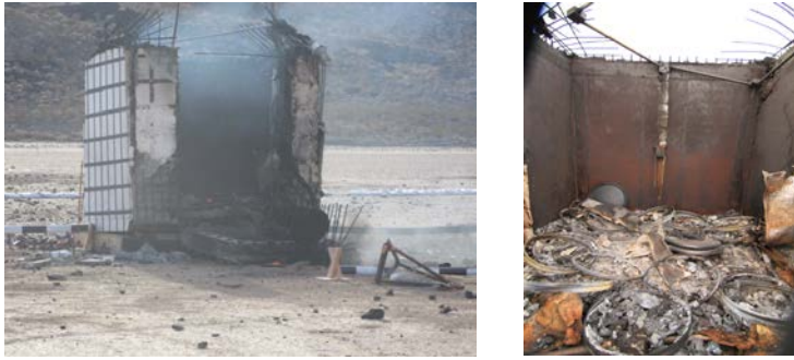
Figure 6 Initial setup (top) and results (bottom) from test with 540 kg M1 propellant (each barrel initiated). (Farmer, et al., 2015).
