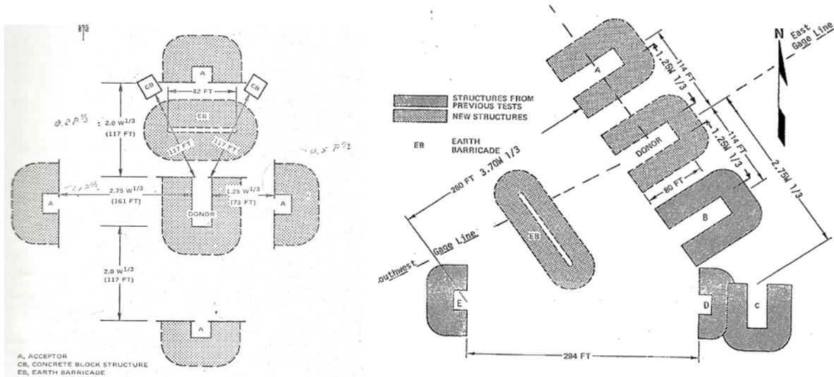
Figure 9. Layout of the Eskimo I magazine separation test [Weals, 1973] (left), and Eskimo III test [Zaker, 1976] (right). Separation distances and charge weights in US units.
