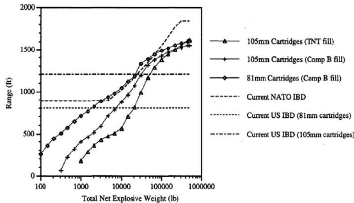
Figure 19. Estimates of the IBD for SsD1.2.1 based on tests with 105 and 81 mm cartridges [Swisdak, 2002] in US units.
