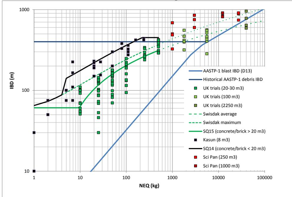
Figure 17. Debris IBD as in Figure 15, with data from Sci Pan trials added.
