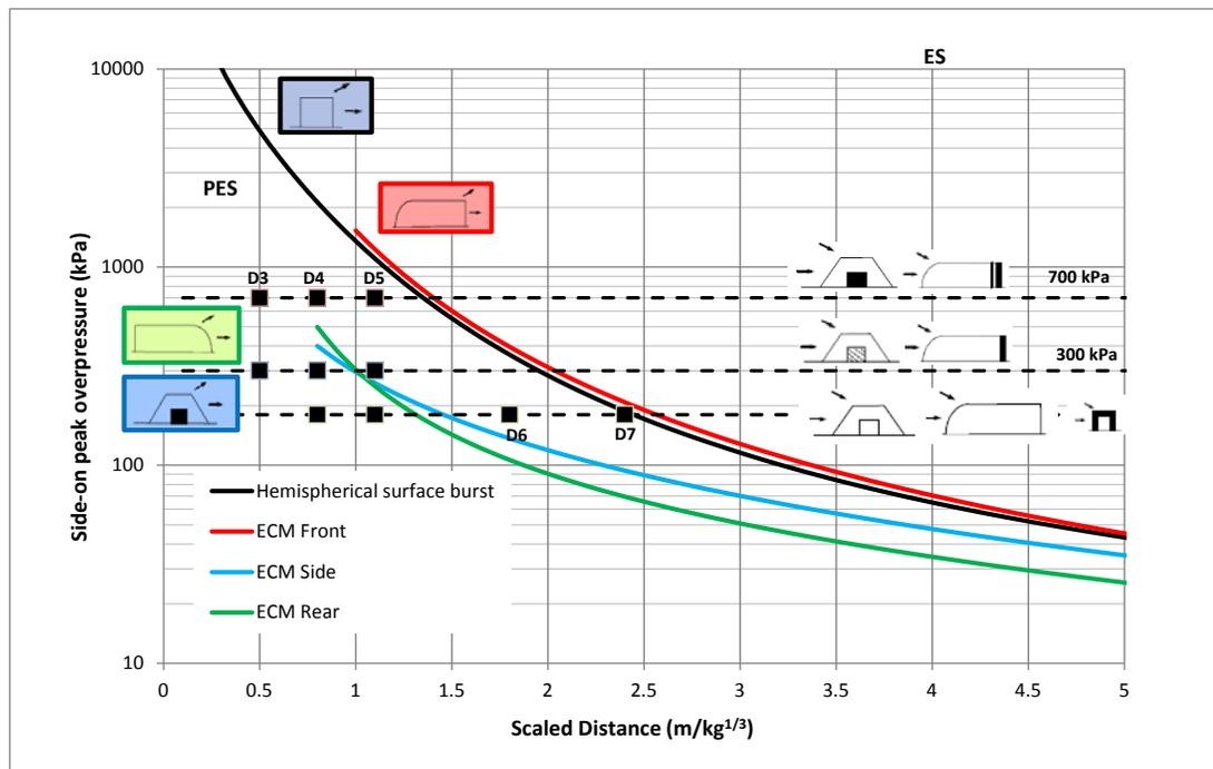
Figure 10. The side-on peak overpressure as a function of scaled distance for a HSB, and for the front, side and rear of an ECM. IMDs for side and rear exposed ECMs are also shown together with design criteria.
