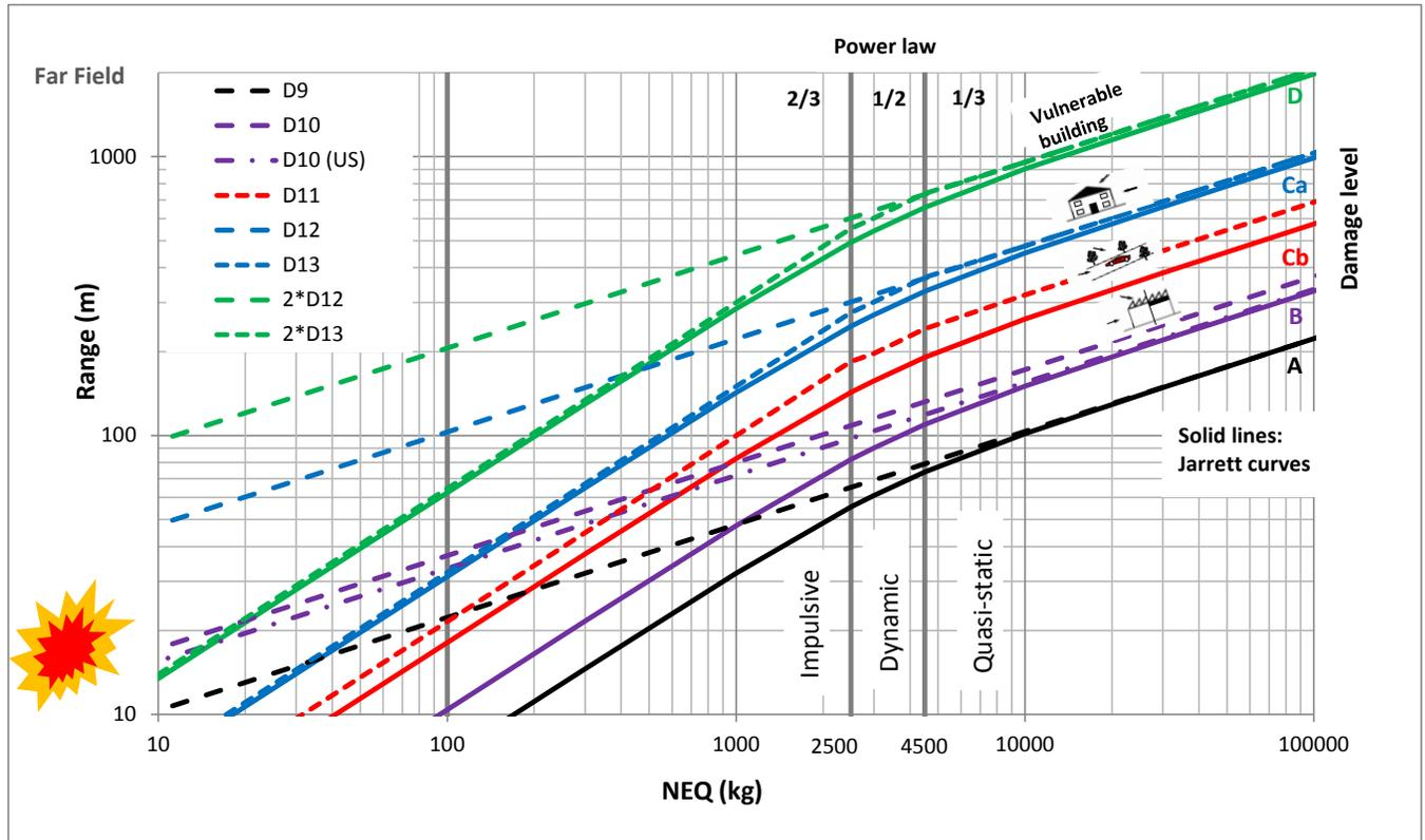
Figure 4. ACR to various damage levels (solid lines) plotted together with a number of HD1.1 Blast QDs from AASTP-1 (dashed lines).
