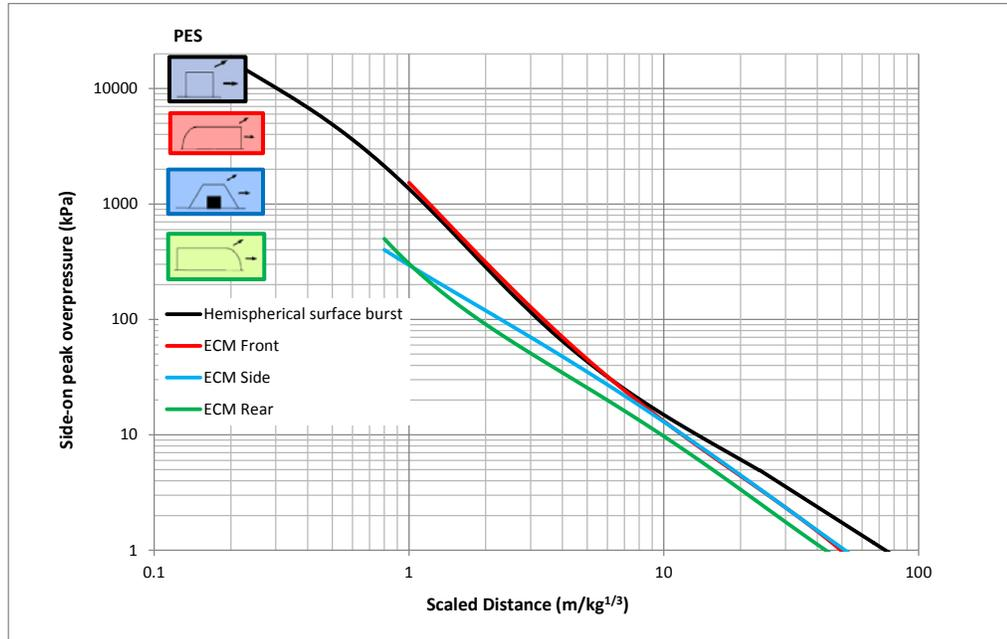
Figure 5. The side-on peak overpressure as a function of scaled distance for a HSB, and for the front, side and rear of an ECM.
