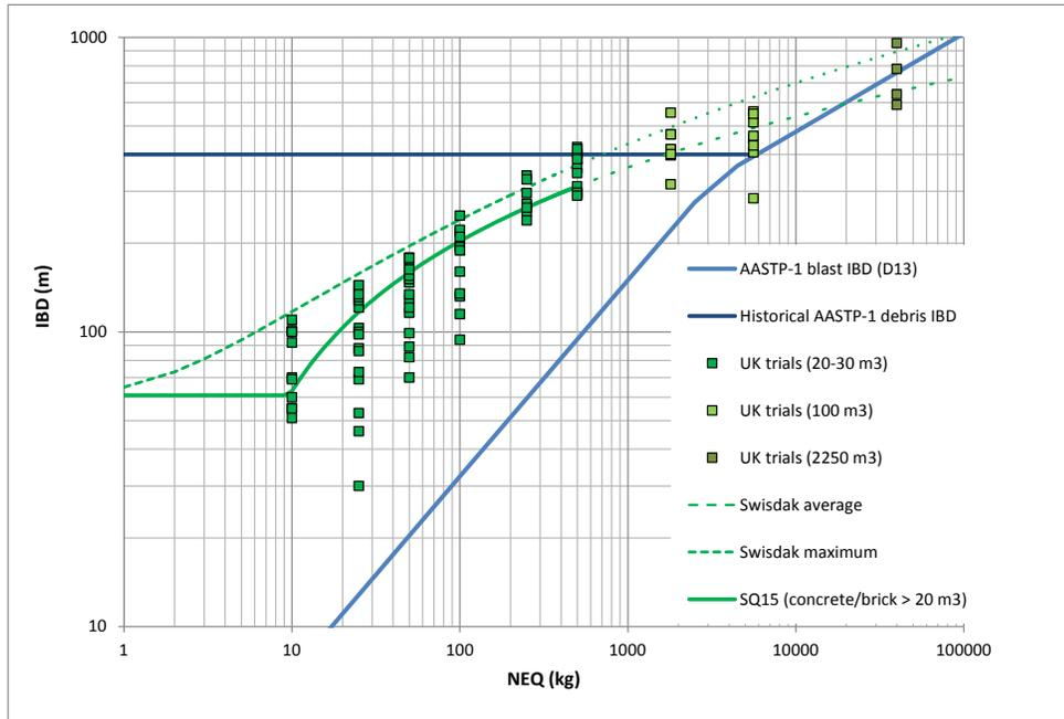
Figure 15. Debris IBD versus NEQ for UK trials together with a datafit by [Swisdak, 2002].
