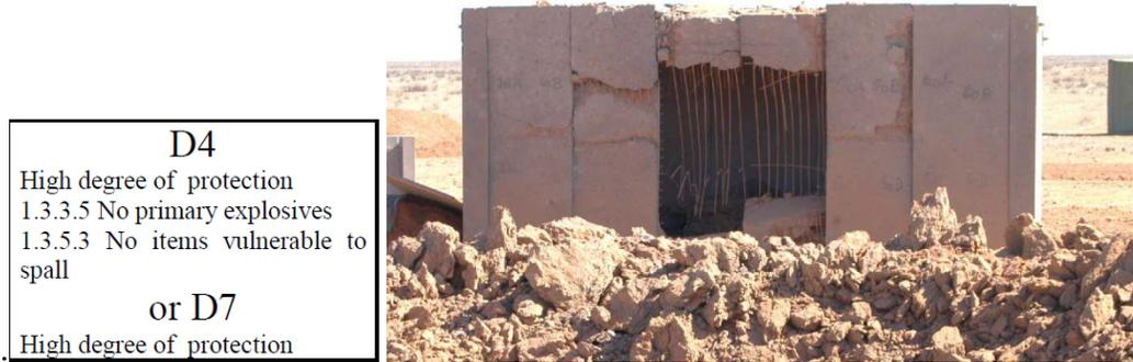
Figure 11. Two options for the IMD towards ES which are protected by barricades from debris and fragments (D4 and D7), but are vulnerable to blast (left). Wall collapse of a Modular Ammunition Magazine at D4 [Van Wees et al., 2006].
