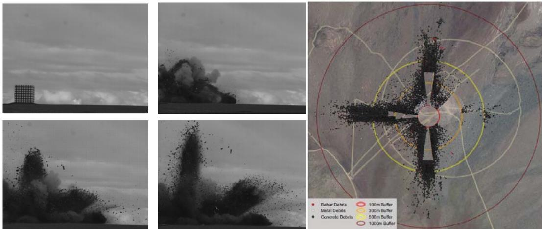
Figure 13. Left: side view of debris throw after detonation of 6.9 kg TNT equivalent in an 8 m<sup>3</sup> RC Kasun structure [Grønsten et al., 2009]. Right: top view of debris throw pattern after detonation of 3,000 kg TNT equivalent in a 250 m<sup>3</sup> RC structure [Anderson et al., 2015].
