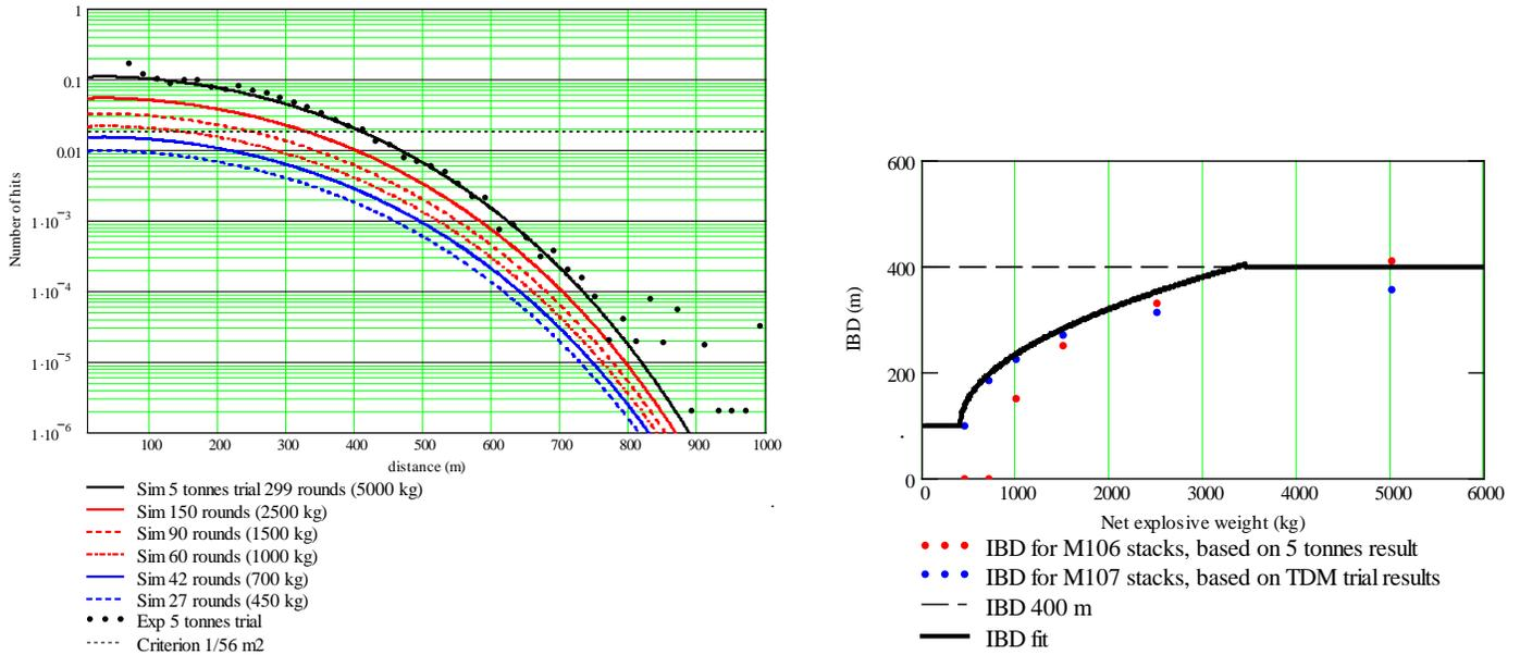
Figure 18. Left: Simulation of 5 tonnes trial together with experimental data. Right: Extrapolation of IBD to other NEQ together with FD8 [Anderson et al., 2008].
