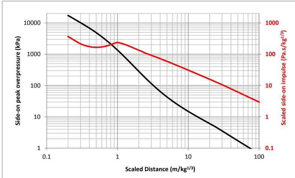
Figure 3. The side-on peak overpressure and scaled side-on impulse as a function of scaled distance for a hemispherical surface burst
