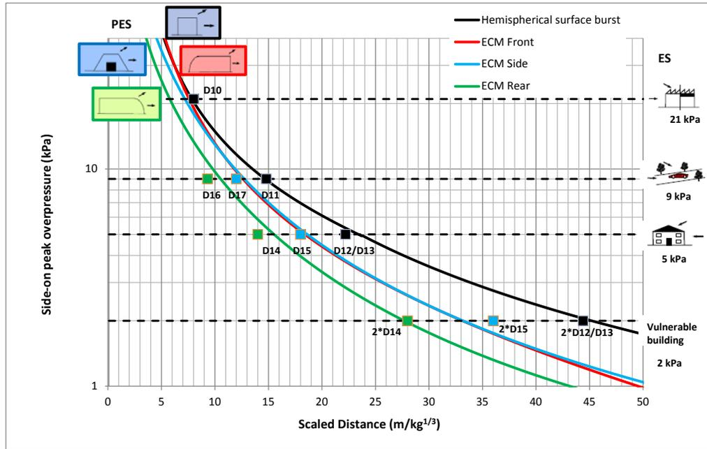
Figure 6. The side-on peak overpressure as a function of scaled distance for a HSB, and for the front, side and rear of an ECM.
