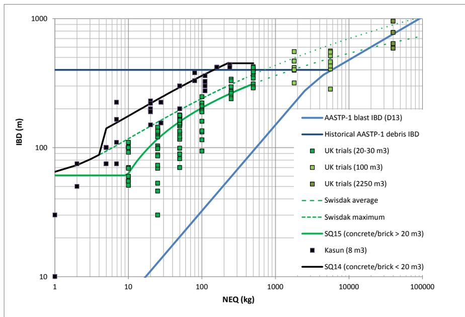
Figure 16. Debris IBD as in Figure 15, with data from Kasun trials added.
