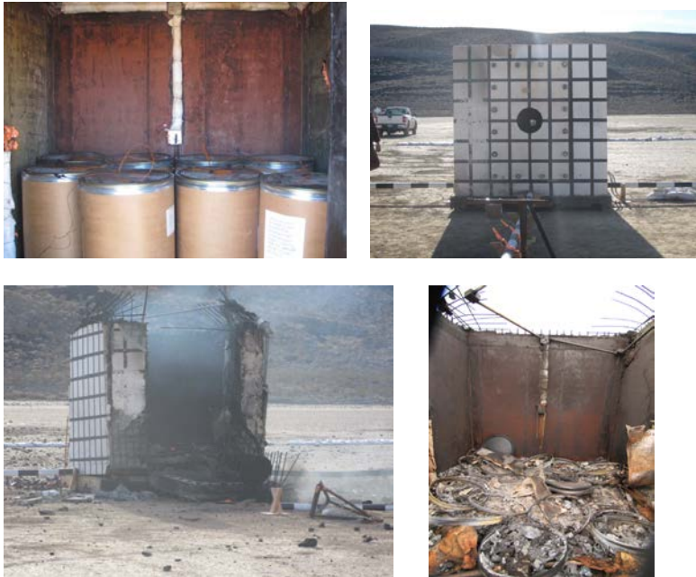
Figure 12. Initial setup (top) and results (bottom) from test with 540 kg M1 propellant (each barrel initiated) [Farmer, et al., 2015].
