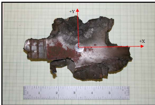
Figure 2. Fragment found at 1824 m after sub-detonative response of artillery shell [Baker, 2009]
