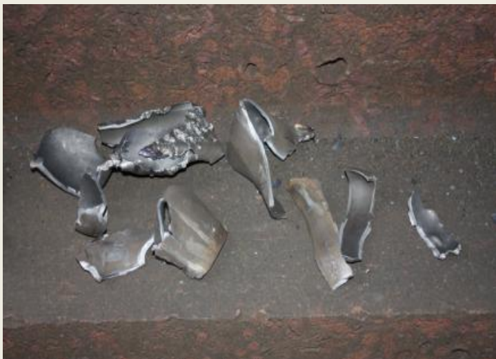
UN Test 2(a) Propellant Fragments (Deflagration)
