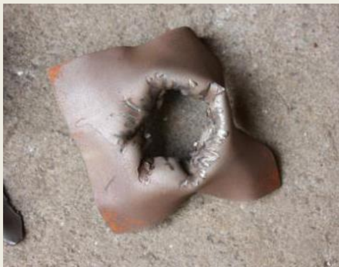
UN Test 2(a) Propellant Witness Plate (holed)
