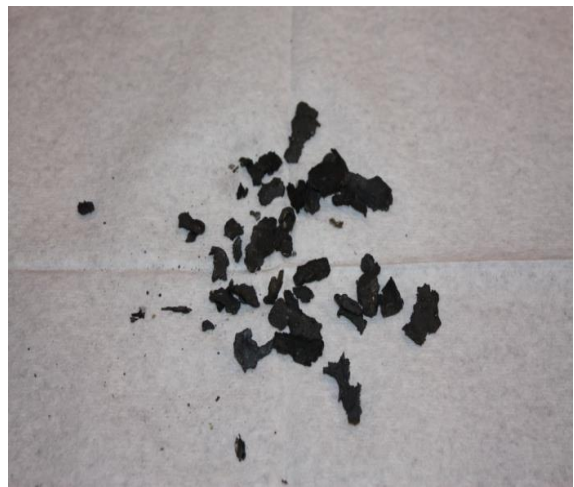
Figure 4: Typical Detonation Fragments
