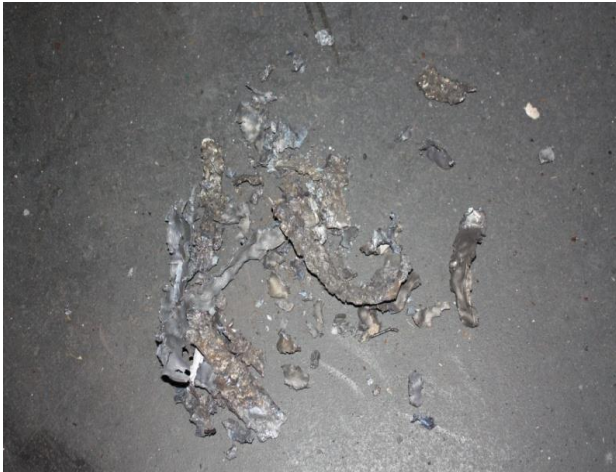
Figure 13: M9 Flake Tube Fragmentation
