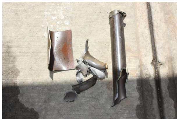
Figure 2: Water UN Test 1(a) Results
