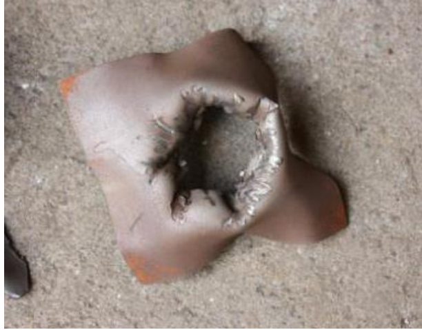
Figure 5: UN Test 2(a) Witness Plate (holed)
