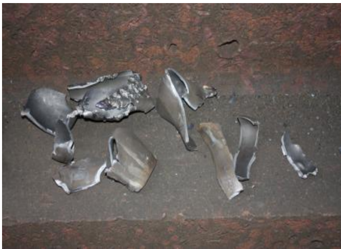
Figure 3: UN Test 2(a) Propellant Deflagration Fragments
