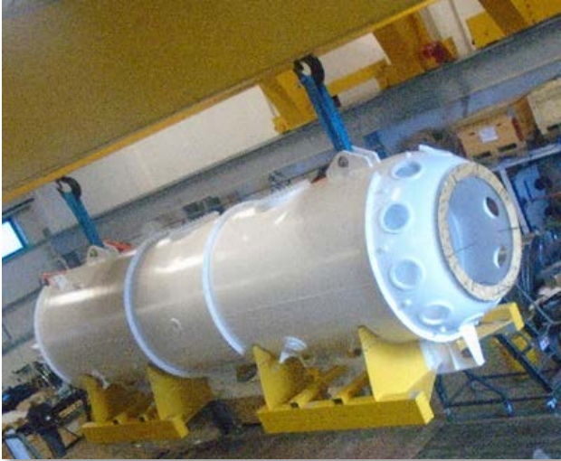
Pressure Vessel Ready for Final Assembly
