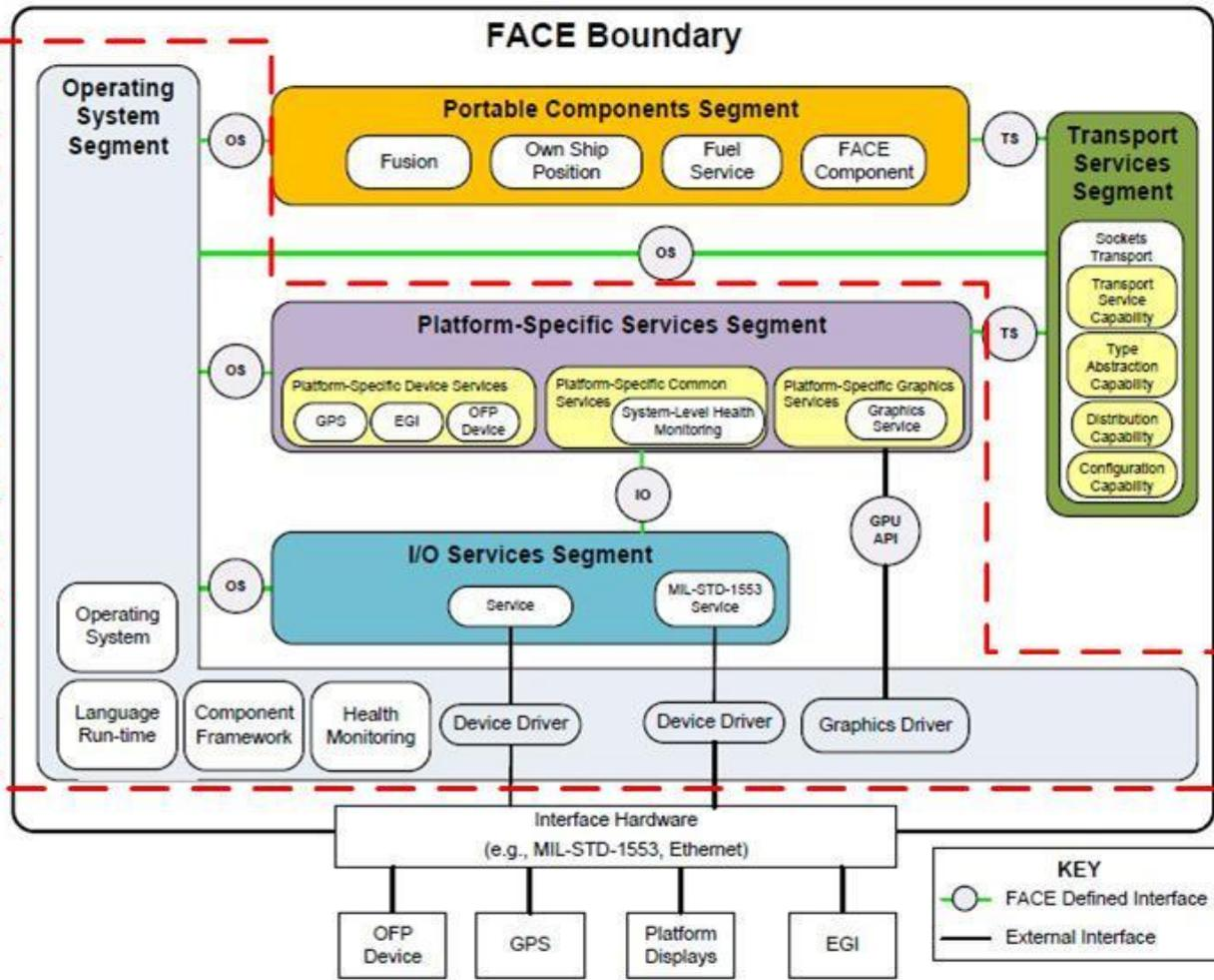
SOSA Software Runtime Environment Interface (REI) may consist of SOSA application software interface to host system for language run time and calls to operating system services as defined by FACE OSS interface, SOSA platform specific software and low level I/O as defined by FACE PSSS and IOSS, SOSA operating system as defined by FACE (Posix, ARINC 653, C, C++, Java, and Ada)
