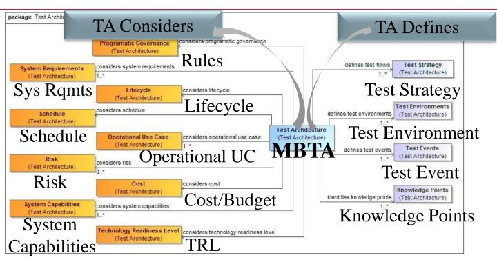
Foundation of the Model Based Test Architecture (MBTA)
