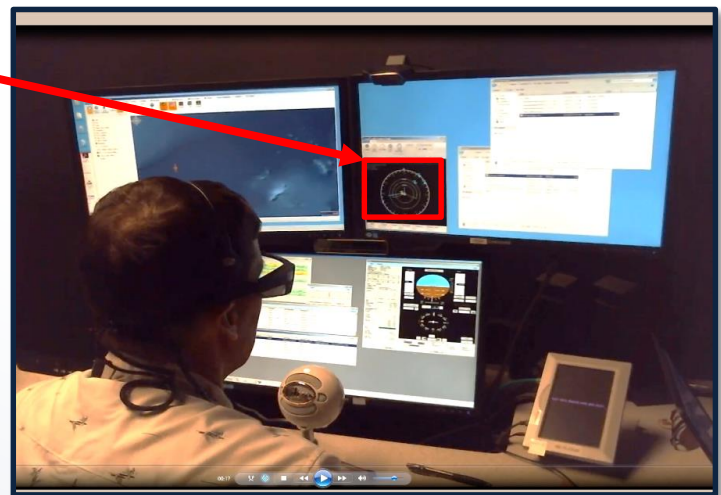
Aircraft Collision Avoidance Display (ACAD) provides the pilot operator with information to aid in self-separation
