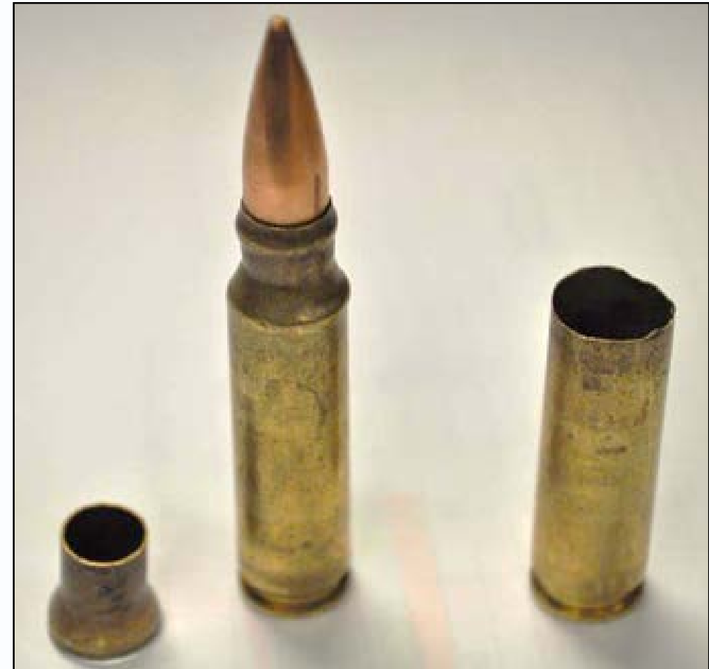
M80 ruptured case and subsequent cartridge which failed to chamber (middle)
