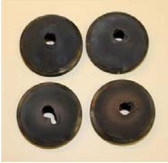
Significant buildup of material on suppressor baffles from endurance firing
