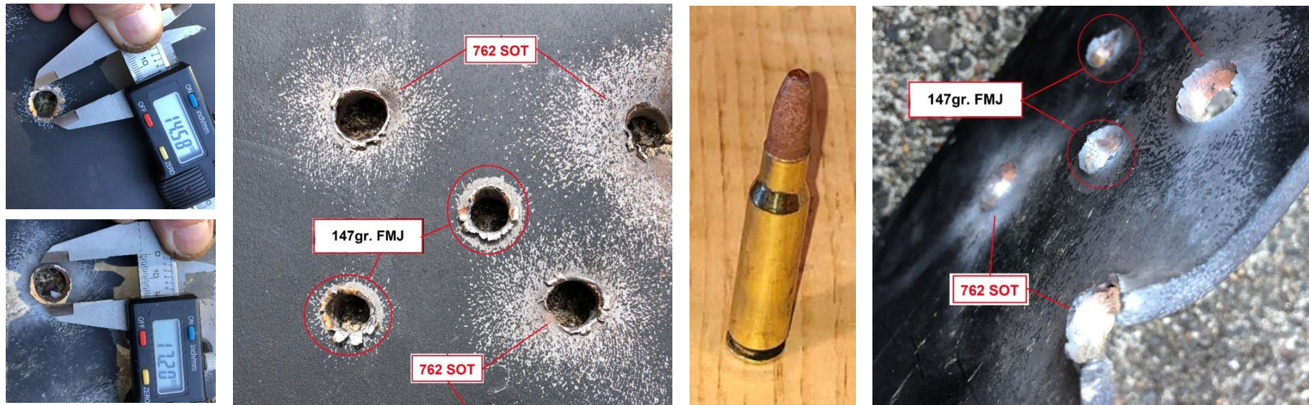
Left To Right Above: 20% Larger Holes In 1/2" Mild Steel With Fragmenting SOT Projectile, Melted Steel And Blast Residue Around Penetrations vs. Bullet Jacket Material Shed From Core With FMJ, 7.62x51mm SOT, Blast And Spall Damage While Producing Four Impact Signatures Which Are Clearly Visible Day Or Night.
