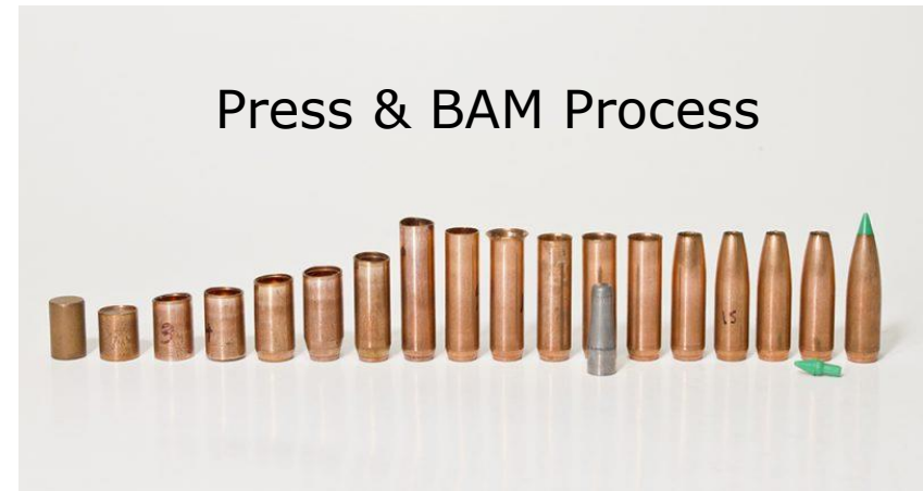
Nosler Ballistic Tip Process Steps Outdoor Hub
