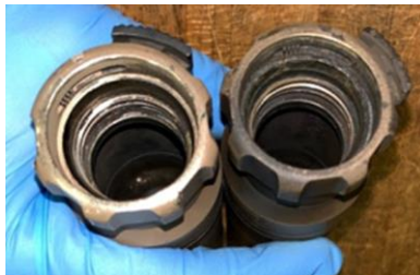
Fired vs Cleaned Suppressor TDA
