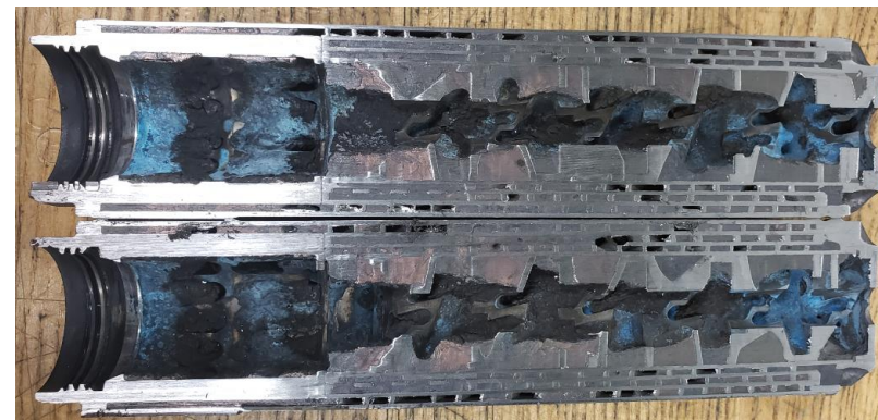
Fouled M110 Suppressor Cross Section
